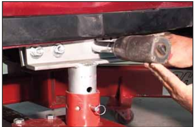
Lower vehicle onto pinchwelds and securely tighten pinchweld bolts.
