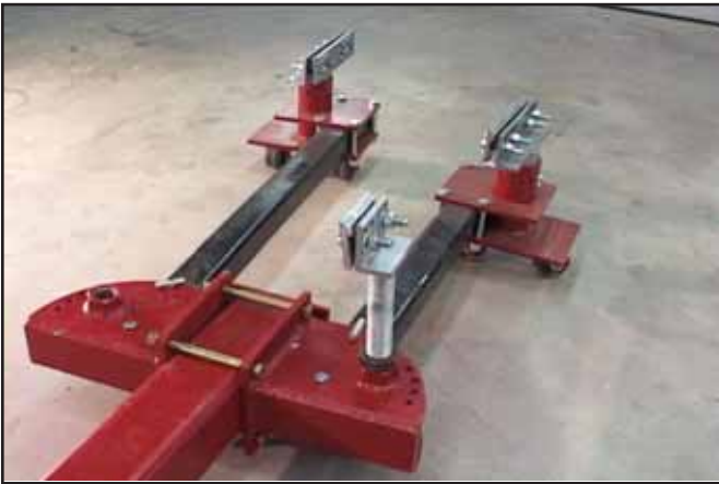
Swing Clamp arms on Versa Puller into closed position. Lock into place with locking pins
