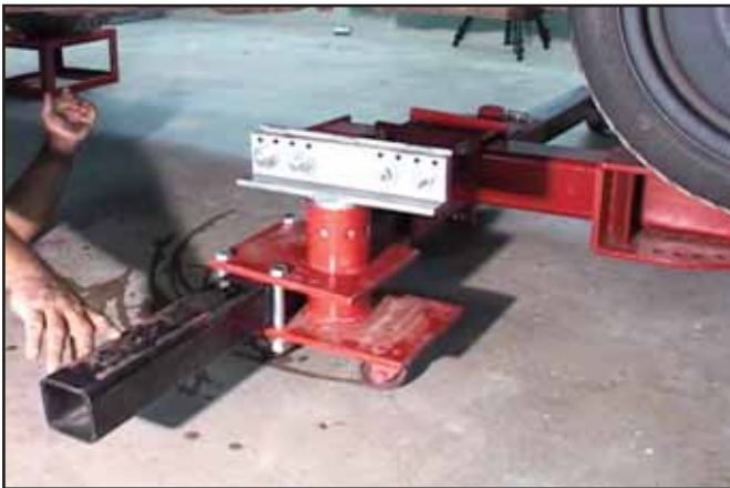
Swing clamp arms out and lock in to place with locking pin.
