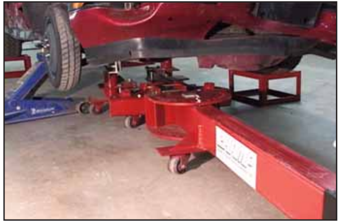
Position Versa-Puller under vehicle.
