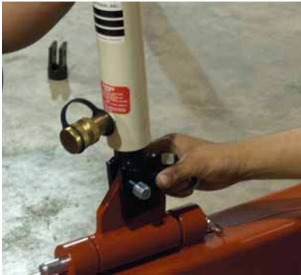
Bolt coupler to Dozer Beam
