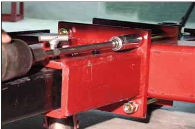
Securely tighten bolts on pinchweld clamp arm mounting bracket.
