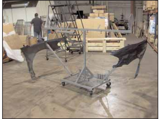
The Universal Parts Stand is ready to be used. Shown holding two fenders
