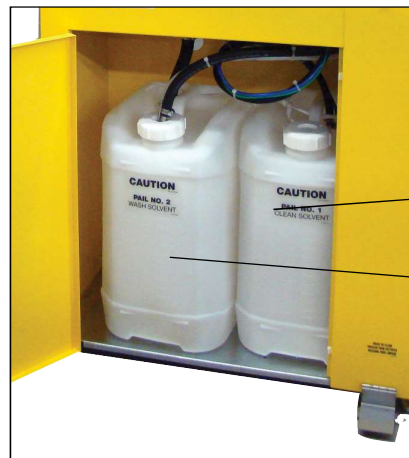
Suction pipe with inlet filter and drain hose is located in wash pail.
