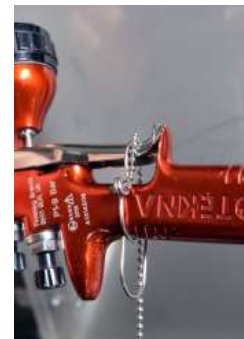
Trigger Lock Spring On Spray Gun
