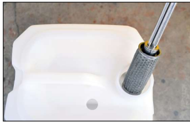
Remove Suction Pipe and Filter
